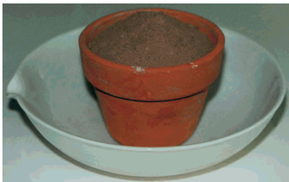
Figure 1. The photo shows the flower pot placed in a porcelain beaker. The flower pot is filled with dry sand and sodium before the water is added into the beaker.
